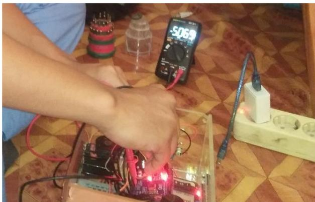
Gambar 2. Tegangan *output* stepdown.
