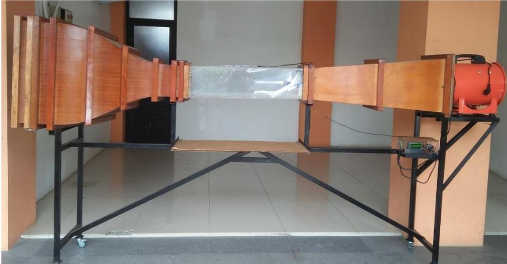
Gambar 1. Open circuit wind tunnel tipe subsonic.
