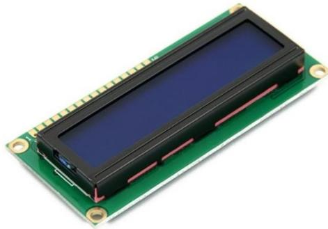
Gambar 8. LCD Display 16 × 2.
